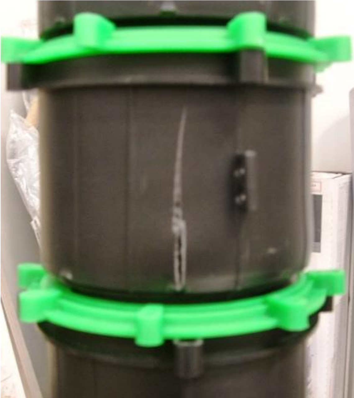
Photograph No.2 Results of Axial Load Test on Specimen #1
