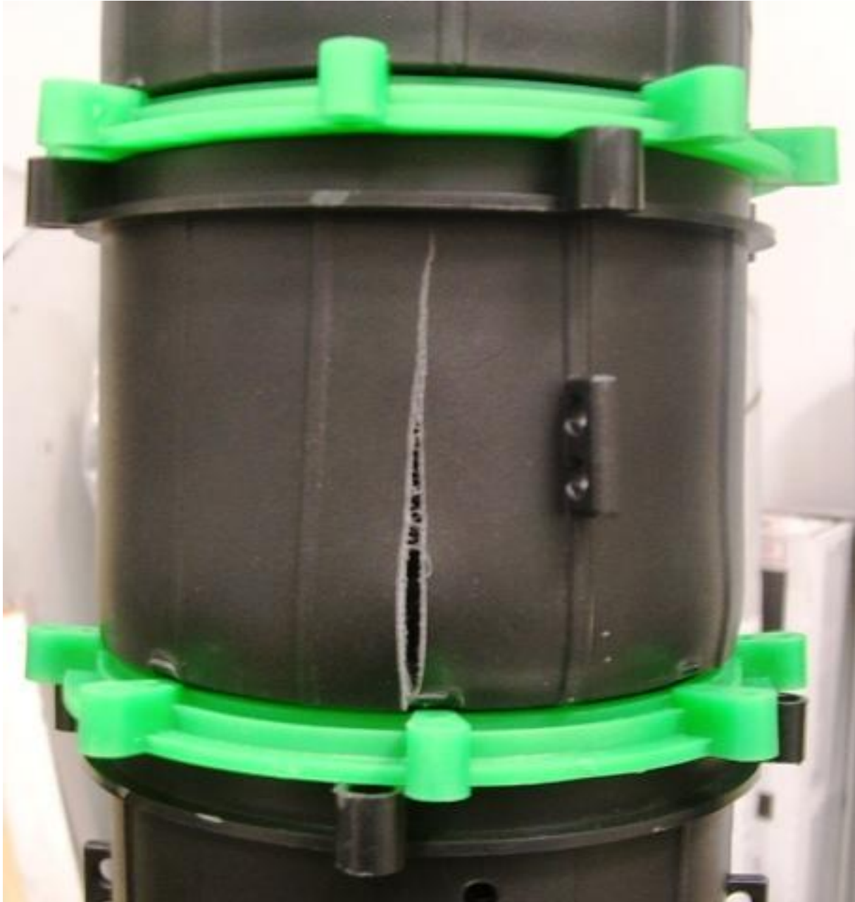
Photograph No.4 Results of Axial Load Test on Specimen #3
