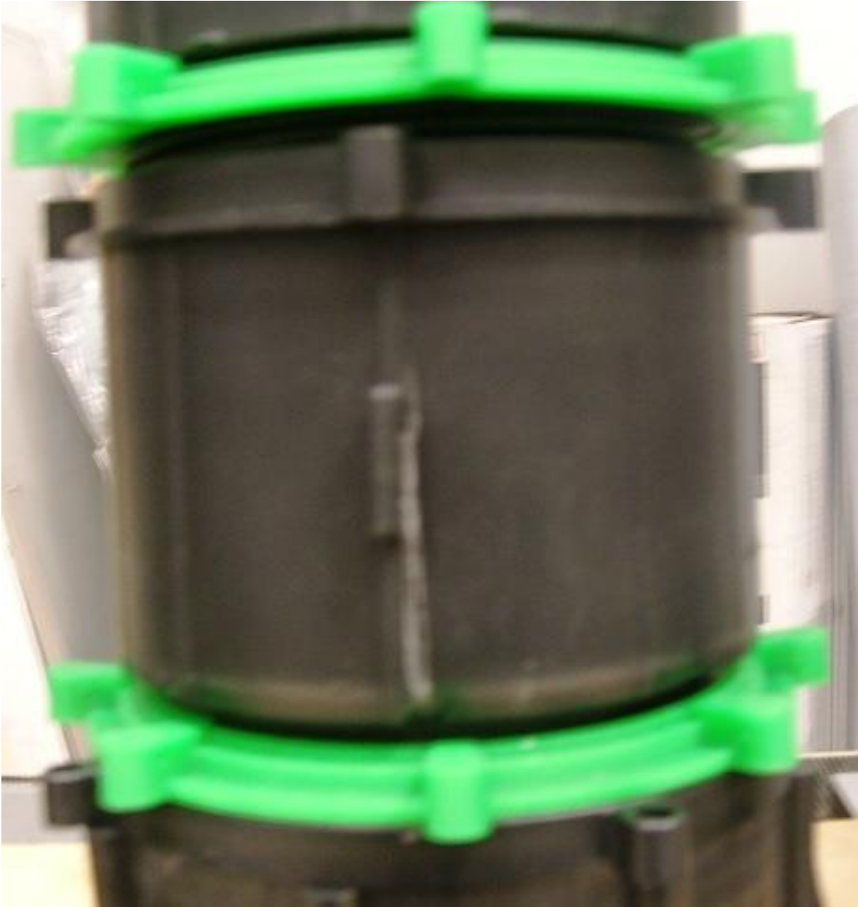
Photograph No.3 Results of Axial Load Test on Specimen #2
