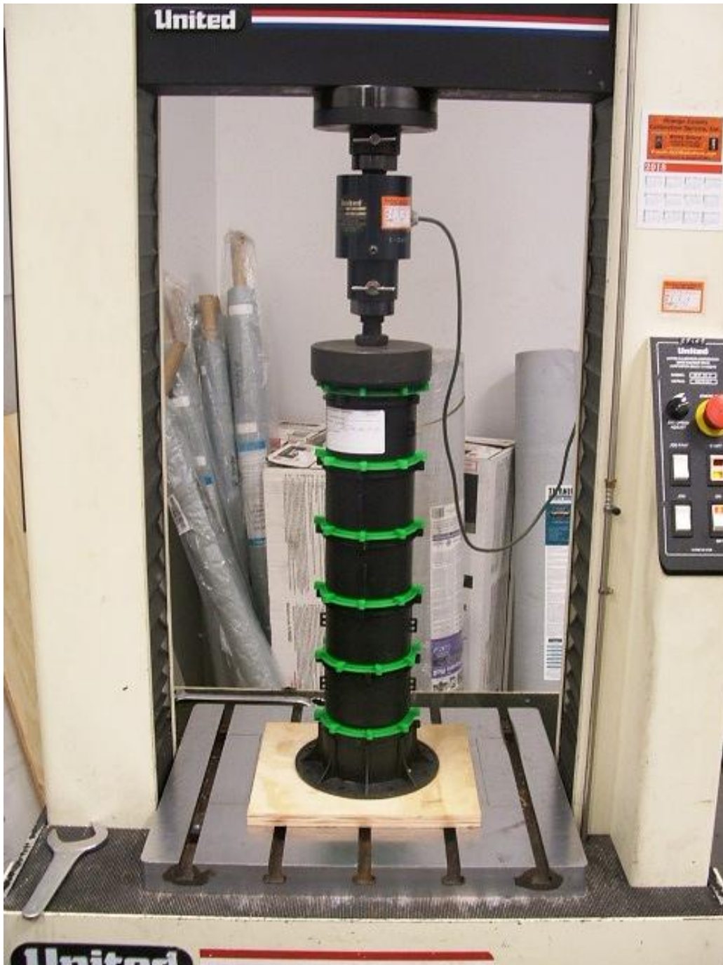
Photograph No.1 22" Pedestal Axial Load Test Set-up
